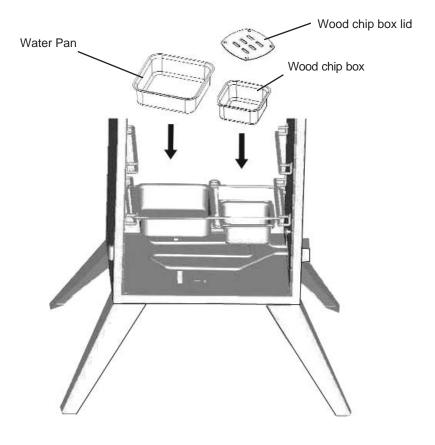
Place water pan and wood chip rack on bottom side racks.
